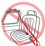
Lap Belt with Motorized Shoulder Belt
